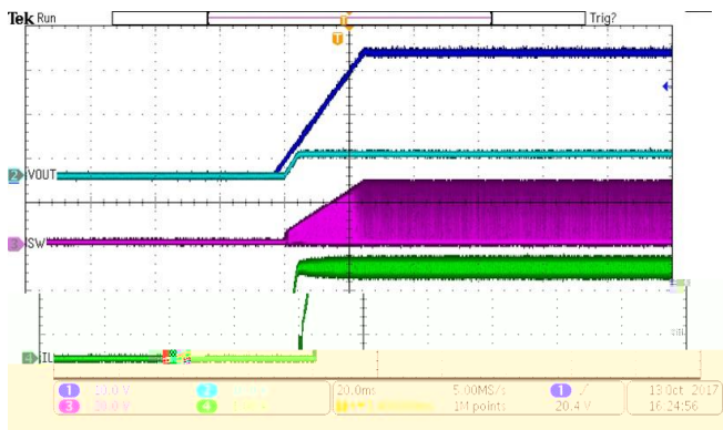
Figure 17. Power Up VIN=24V, VOUT=5V, IOUT=2A
