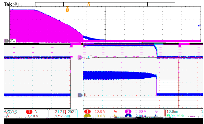
Figure 13. Power Down, IOUT=3A
