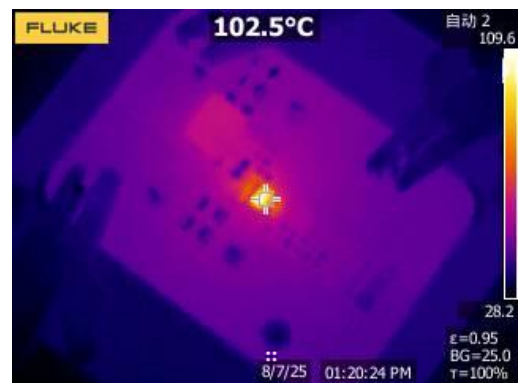
Figure 21. Thermal, 12VIN, 5VOUT, 3A
